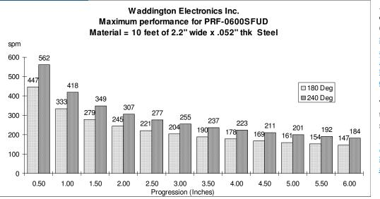
All calculations are based on <u>real world conditions</u> (as best <u>as we can</u> <u>simulate on a computer).</u> <u>Allowances are made for</u> <u>loop size and material</u> <u>thickness, width, and</u> <u>density.</u>
