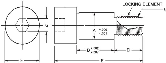
Socket Shoulder Screws are held to much closer tolerances than on standard Stripper Bolts. **The "B" dimension is always a plus to eliminate the binding on movable plates.** The "A" dimension is held closer for bearing-type locating. You'll get more positive holding power and greater turning leverage. Ideal for all sliding mechanisms. Nylon locking element is incorporated in all Jergens Shoulder Screws.
